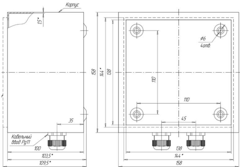
**Fig 5. Repeater UDR-6(x)-blk installation dimensions**
