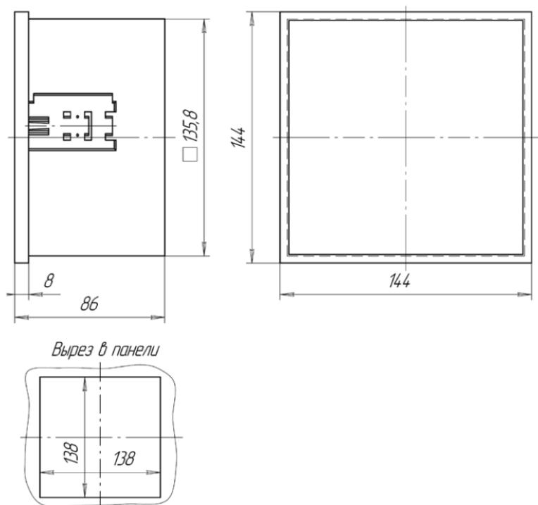
**Fig 4. Repeater UDR-6(x)-fl installation dimensions**
