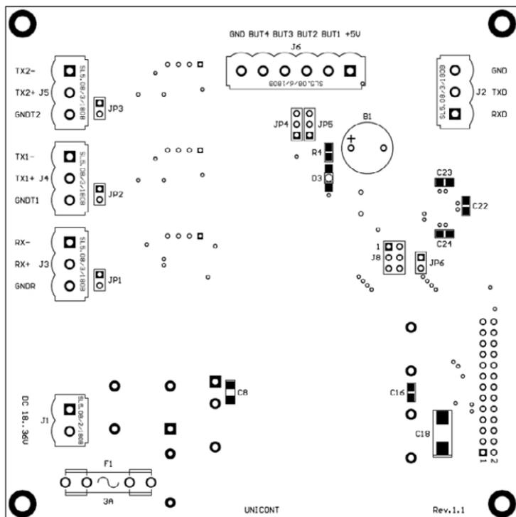
**Fig 3. Arrangement of terminals on printed circuit board.**
